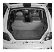
To open the hatchback press the release button in the rear of the vehicle and open upwards. Beneath the rear storage area you will find a rear deck lid. To open, you must push the rear seats forward and lift the lid (Fig 1). Inside you will find the motor, the contactors, the battery charger and the motor controller. These are often very hot, even during charging. DO NOT TOUCH them. If you
